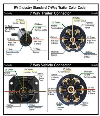
Wire the Trailer Brake Controller as shown, Install a 20 Amp Auto-Reset Breaker and 12 Ga wire.
